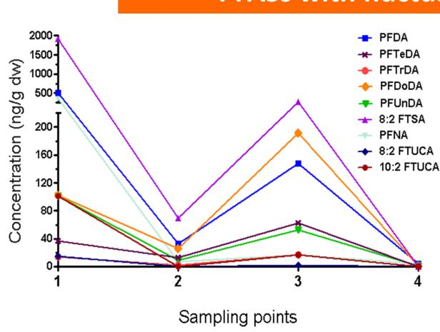
Severe concentration increase for the long chain PFCASs (≥ PFNA) and FTs (8:2 FTUCA and FTSA, 10:2 FTUCA) near the filter press. This is likely related to accidental spillage of dry sludge.
