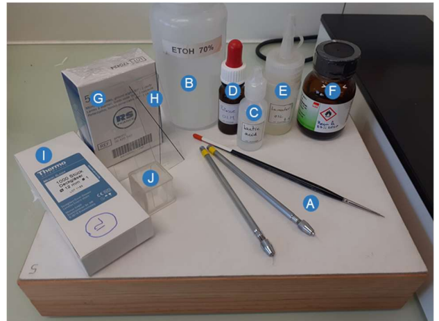
Figure 3. Mounting material. A: brush and micro-pins; B: ethanol (10%, 70% and 95% needed); C: 30% lactic acid; D: 0.1M KOH (NaOH also convenient); E: lavender oil; F: Canada balsam; G: microscope slides; H: centering template made from microscope slide; I: 12mm diameter rounded cover slips; J: 20x20mm square cover slips.
