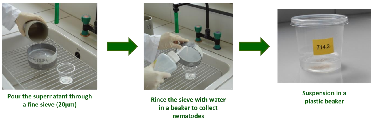
Figure 6. Transferring the contents of the 20 \mu\text{m} sieve containing the extracted nematodes to a plastic beaker. Suspension can be stored and observed through the beaker in the stereomicroscope (Picture ANSES - Nematology Unit, France).
