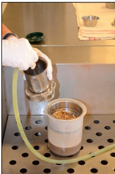
Figure 5. Rinsing of blender beaker after mixed content was poured on an 850 \mu m sieve on top of a 1 L beaker.
