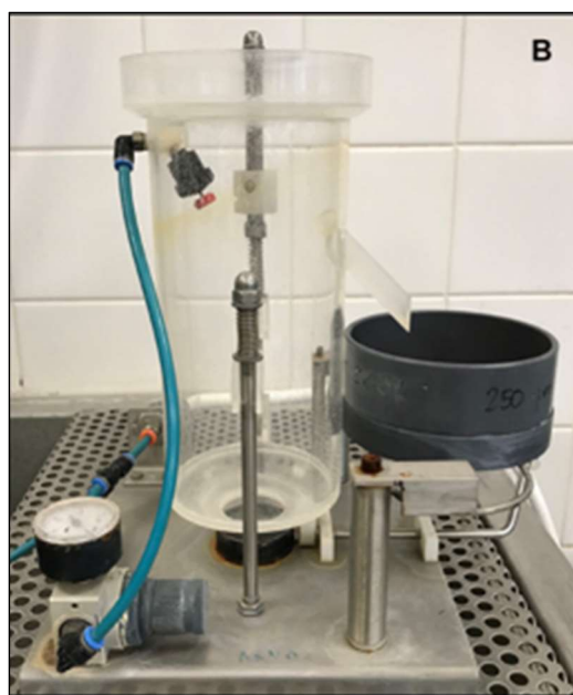
Figure 6. Arvo can 3 equipment to clean the extract obtained with the Schuling centrifuge.
