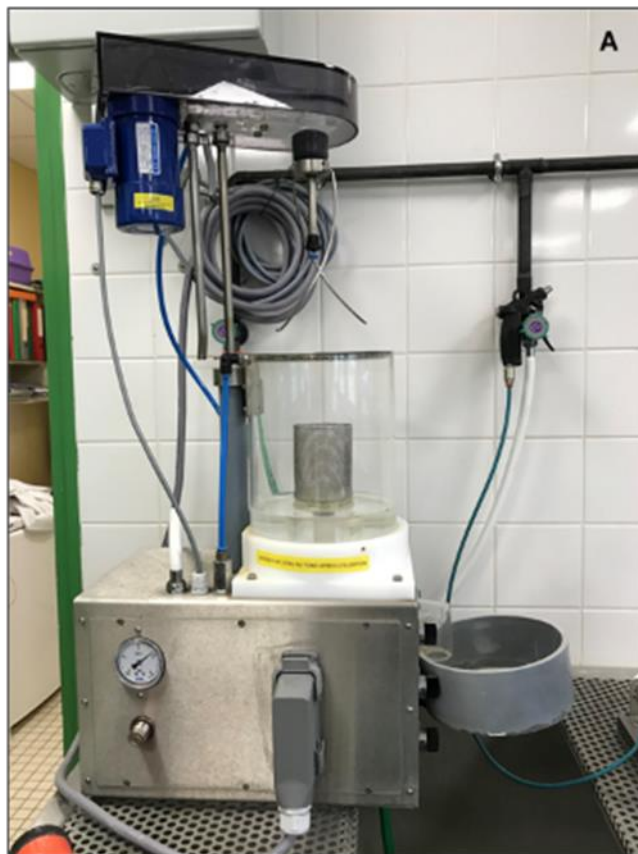
Figure 2. Schuiling centrifuge to extract cysts from soil samples at ANSES-LSV (Picture ANSES-LSV, France).
