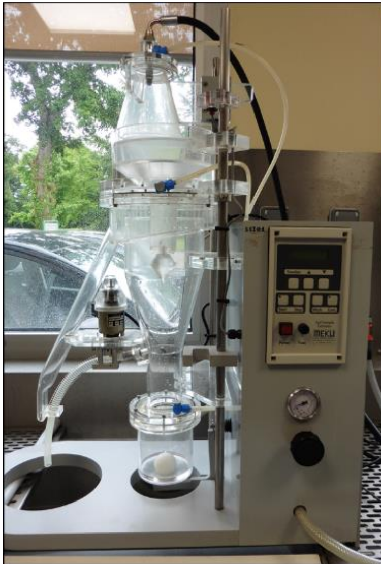
Figure 3. Semi-automated Seinhorst Meku Elutriator to extract cysts from soil samples at ANSES-LSV (Picture ANSES-LSV, France).
