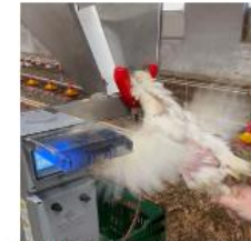
Figure 6: Birds head is introduced between the tongues of the stunner.
