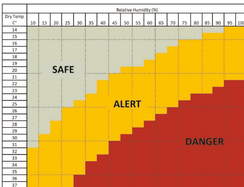
Figure 1: Thermal Comfort Zones for broiler transport defined by Apparent Equivalent Temperature by Mitchell et al. (2004, 2005, 2006 in EFSA, 2022)
